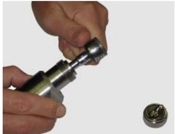
2. Loosen and remove the nozzle (3) with socket wrench, size 7.
