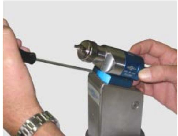
2. Fixing automatic gun AGR-09 mini and the „stud with tip“ with a hexagon socket head wrench, size 4
