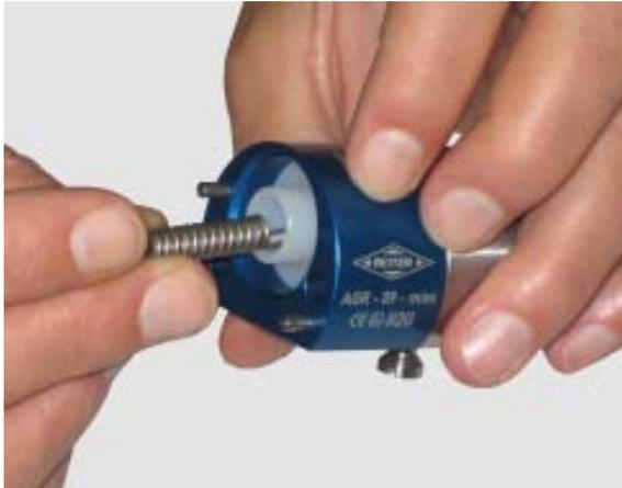
10. Push the small spring (16) onto the spring pin.
