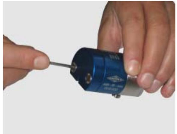
13. Tighten the screws (18) to a torque of 4,5 Nm.
