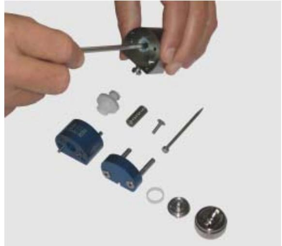
If the hexagon socket head wrench does not grip, pry the needle set (9) out with a turn screw.
