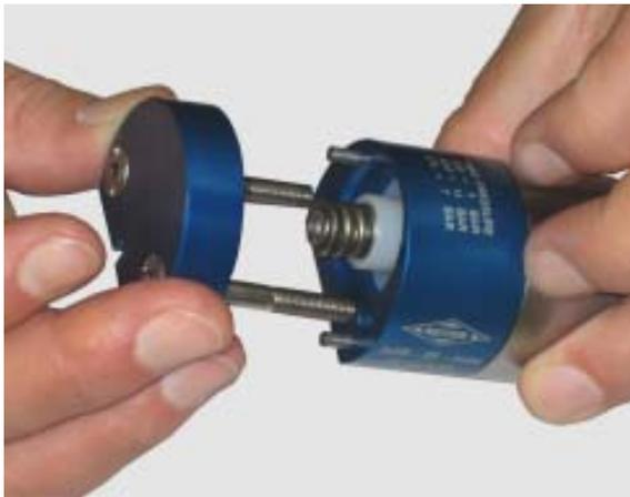
12. Place the end plate (17) with the countersunk screws (18) on the head holder.
