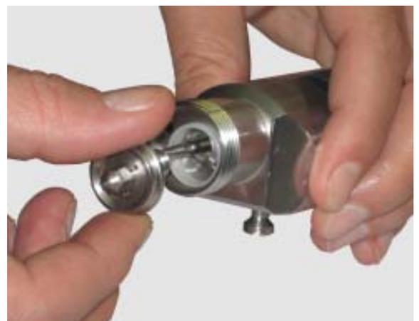
18. Attach and tighten the nozzle (4).
