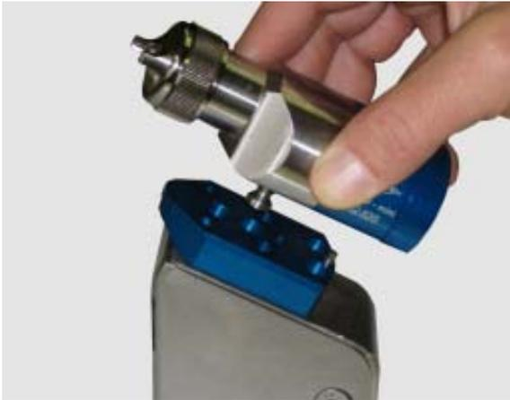
1. Fixing gun on the intermediate plate.
