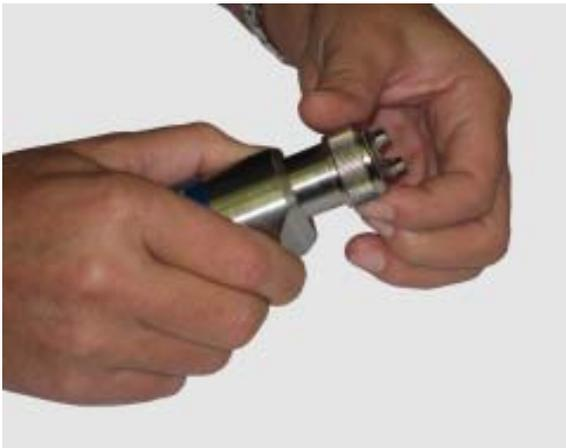
1. Screw on retaining ring (1) and remove air cap (2).
