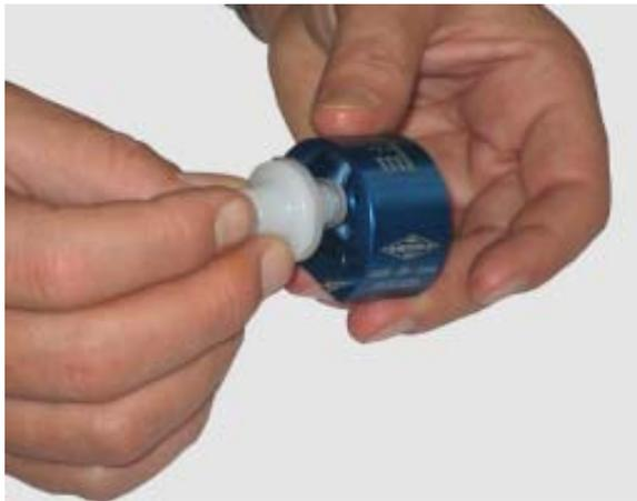
6. Grease the piston (12) and insert it into its position in the head holder (11).
