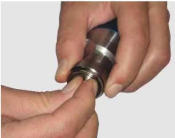
21. Tighten the air cap with the retaining ring (1).
