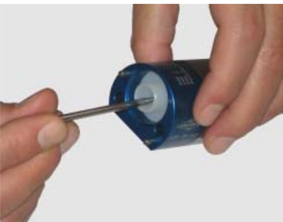
8. Grease the paint needle (13) and stick it into the piston (12).
