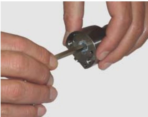
2. Screw the needle set (9) into the head (8) with a size 6 hexagon socket head wrench, to a torque of 0,8 Nm.
