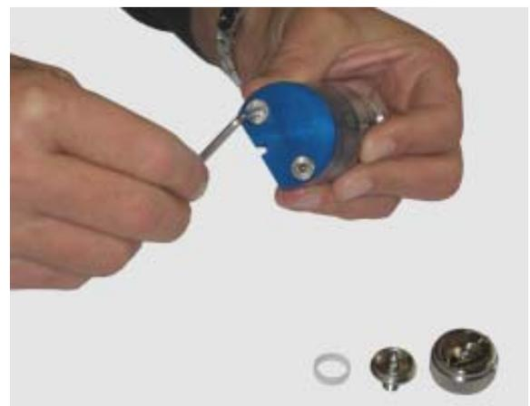
4. Loosen two countersunk screws (18).
