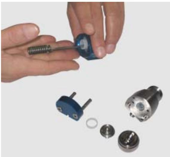
7. Remove the two springs (15 and 16), spring pin (14) and paint needle (13).
