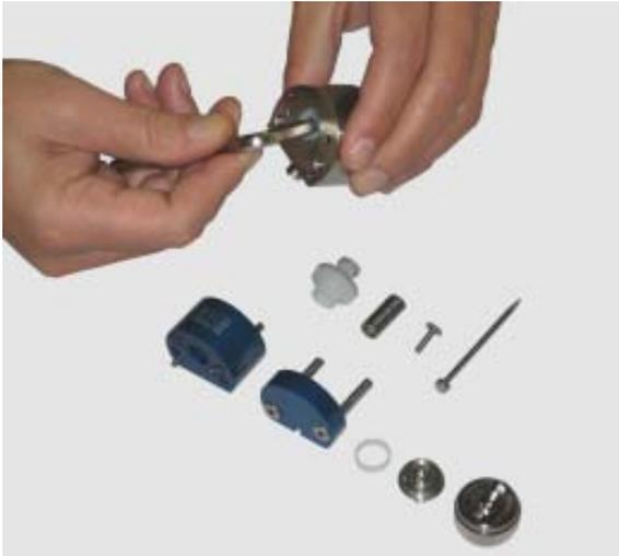
9. Unscrew the needle set (9) with a hexagon socket head wrench, size 6.
