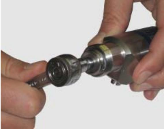
19. Tighten the nozzle to a torque of 10 Nm.
