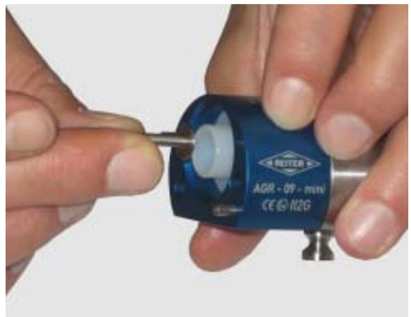
9. Insert the spring pin (14) into the piston.
