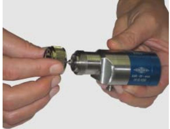
20. Attach air cap (3) with air cap gasket (2).
