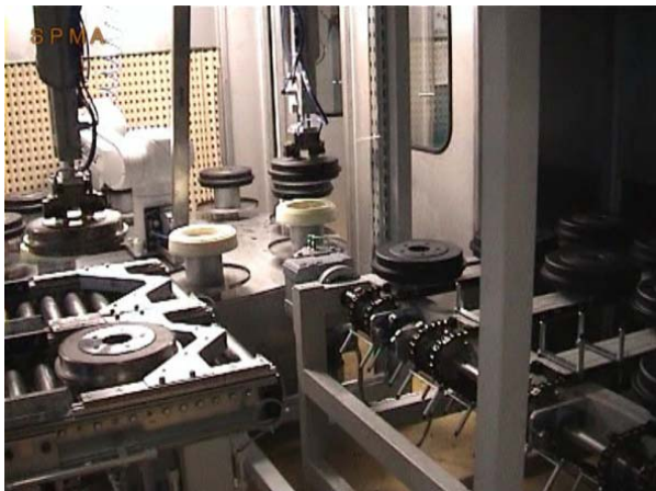
Round table machine integrated in fully automated production line
