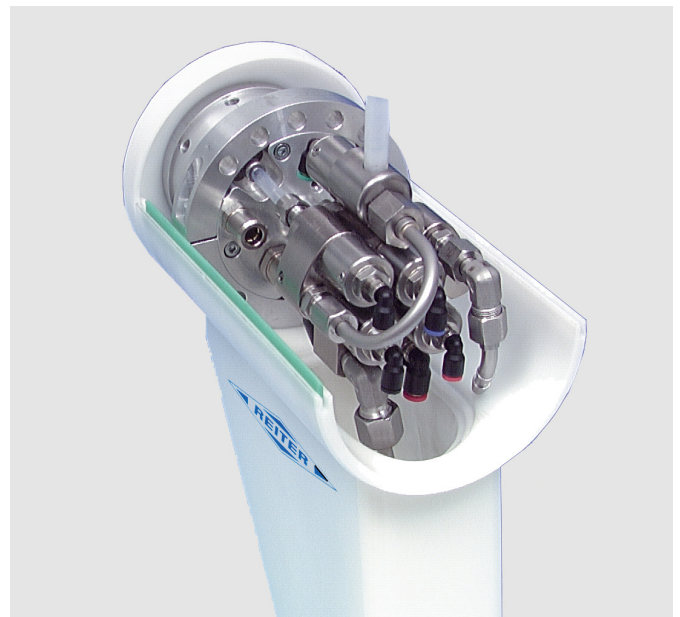
Material and control hoses are feed through the hollow wrist and arm of the robot to the atomizer couplings.
