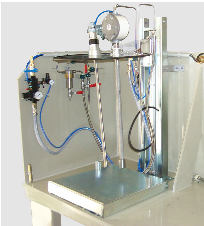
Elevator unit with low level control on insulated desk
