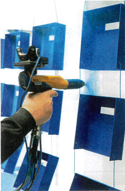
This system can be used to program robots for coating by manually demonstrating the process.
