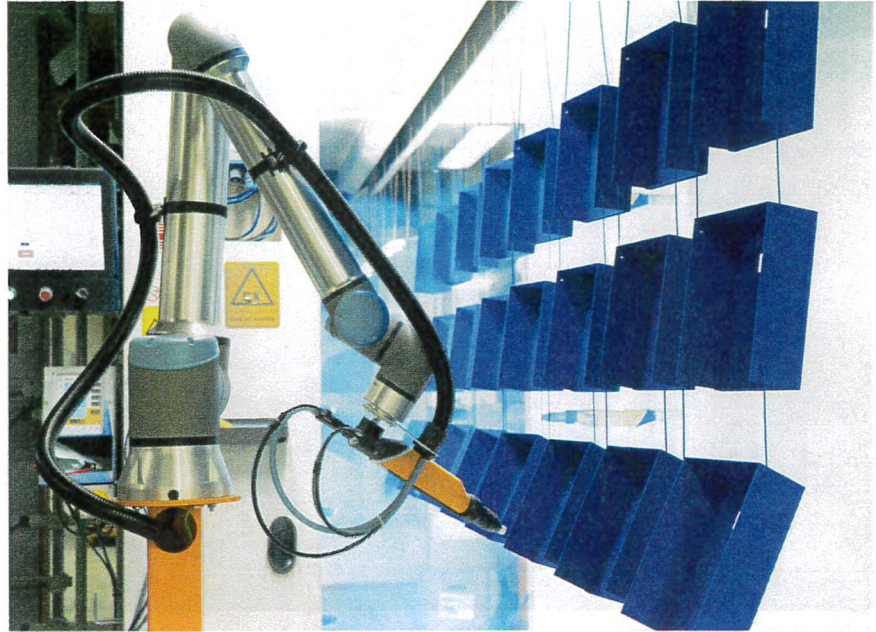
This system can be used to program robots for coating by manually demonstrating the process.
